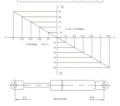
Gas springs are manufactured at a temperature of 20°C
