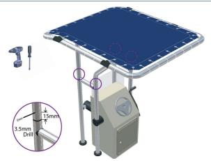
**C.** Attach the **CANOPY SECTION** to the **BASE SECTION**. Secure permanently using self tapping screws (supplied) (As shown in the diagram)
