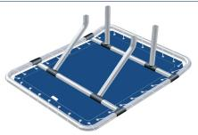
**E.** Lay out the **canopy fabric** topside down and place the inverted frame over it. Lace **nylon cord** through the eyelets and frames, Ensure its evenly threaded and tight.
