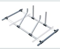
C. Insert the U frames onto the ends of both side frames.
