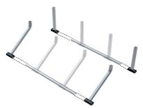
B. Insert side frames into the support poles. The support pole housing the 'T' joiners should be closest to the side frame bend.
